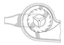
From the above, it is witnessed that the kinetic energy of the wind is striking the blades of propeller in parallel. Due to this construction, there are many disadvantages. First and foremost thing is that it's occupying much space. Due to that, the vehicle is looking awkward in above two cases.
