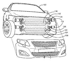
As shown in the figure, the crank wheel assembly is analogous to the rim of the dynamo which will be in contact with the wheel of the vehicle.
