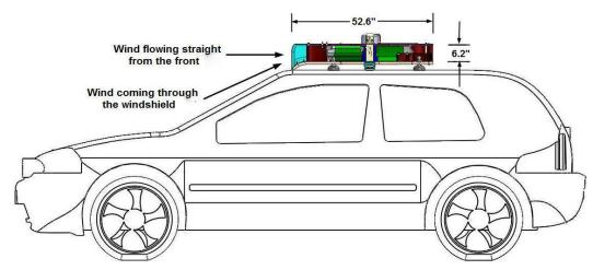
Francis type model of turbine is installed over the roof of the vehicle to drive the dynamo that can charge up the required battery to supply power to the components of the vehicle. Unlike the above two models, it is comparatively better in all aspects.
