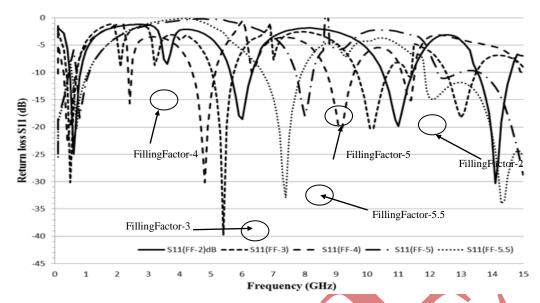
Figure.6. Return loss vs. frequency plot
