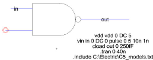
Fig.16. Spice simulation for DC analysis for NAND gate
