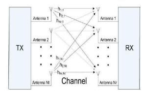
Summation=diag(sigma1,2,r,0,...0). Thus, the MIMO channel can be decomposed into r independent SISO channel has a gain sigma i and a noise factor vi, and assumes the representation. This implies all the efficient signaling and decoding strategies welll investigated in the SISO context could be transferred mutatis-mutandis to the MIMO framework with a minimal effort.
