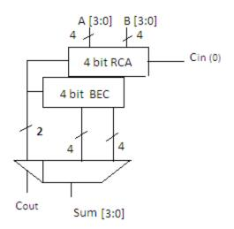
Fig.5. Replacement of RCA with BEC
