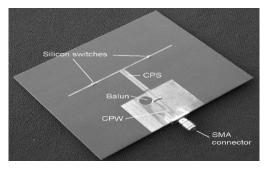
Fig. 5. Photograph of the switched dipole antenna [9]
