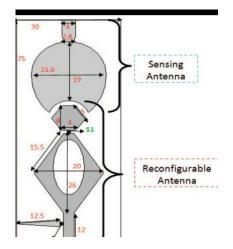
Fig 4. The proposed cognitive radio antenna structure [7]
