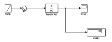
Figure11:Simulink model for Ramp first order without feed back
