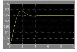
Figure 8 Unit Step second Order System without Feedback
