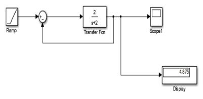
Figure13:Simulink model for Ramp first order with feed back
