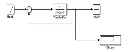
Figure 17:Simulink model for Ramp second order with feed back
