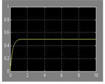
Figure 6 Unit Step Order Systemwith Feedback
