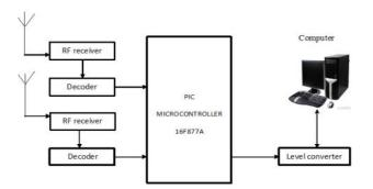
Figure 4 Shows that Block Diagram of EB Section
