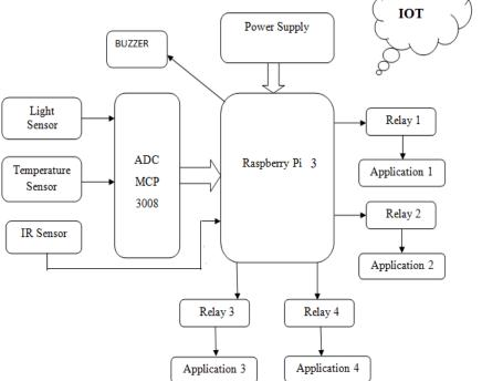
Fig.3 Block Diagram of industrial Automation System by Using Raspberry Pi
