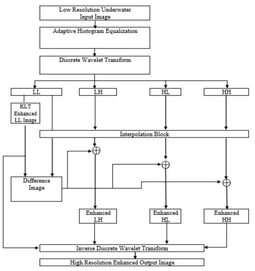
Fig. 1 : Proposed system to enhance underwater images.
