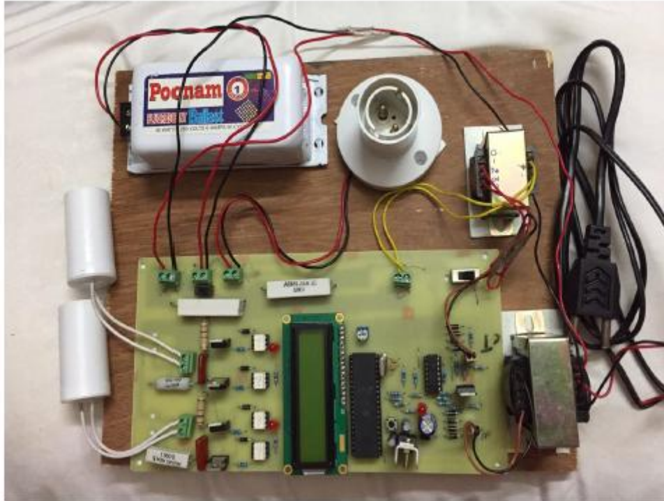
Fig.5. Experimental set up of single-phase SVC
