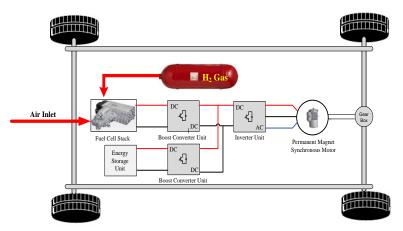
Figure 1. Block Diagram of the Fuel Cell Electric Vehicle
