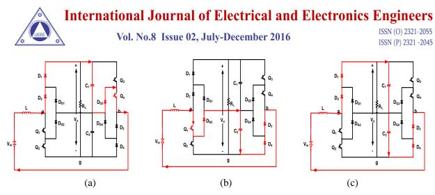
Figure 4. Operation states of suggested Converter. (a)  $D_1$ ,  $D_2$ ,  $Q_4$ ,  $D_{Q3} = ON$  and  $V_{ab} = V_0/2 = V_{C1}$ ; (b)  $Q_1$ ,  $D_{Q2}$ ,  $D_3$ ,  $D_4 = ON$  and  $V_{ab} = V_0/2 = V_{C2}$ ; (c)  $D_1$ ,  $D_2$ ,  $D_3$ ,  $D_4 = ON$  and  $V_{ab} = V_0 = V_{C1}+V_{C2}$
