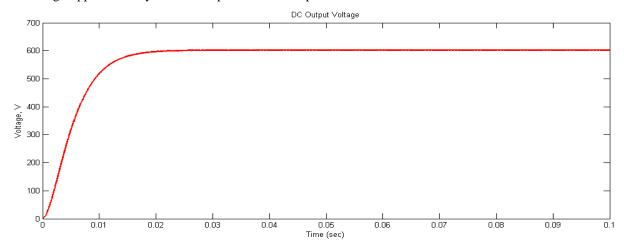
Figure 8. Output voltage of high gain boost converter
