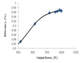
Figure 9. Output power versus Converter efficiency
