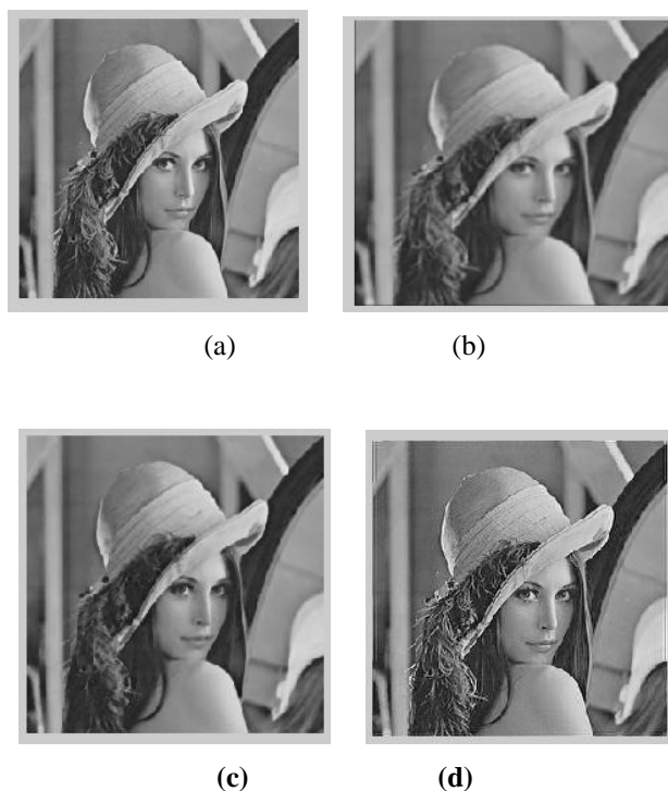
Fig. 2. Samples showing the effect of preprocessing filter (a) The original image, (b) Mean filter (c) Median filter (d) Wiener filter
