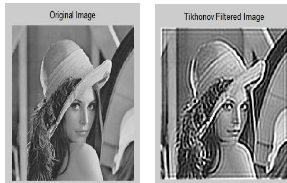
Fig. 4. Result of denoising using Tikhonov model (a) The original image, (b) Tikhonov Filtered image
