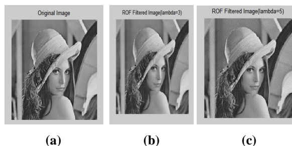
Figure 5. Result of denoising using ROF model (a) The original image, (b) TV using \lambda=3 , (c) TV using \lambda=5 .
