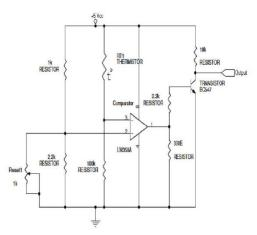
Fig 5. Circuit diagram for temperature sensor
