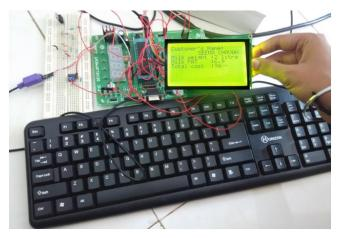
Fig. 4 Interfacing keyboard and GLCD with pic
