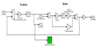
Fig.10: Two Mass Drive Train Model
