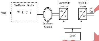
Fig. 4: Proposed Wind Energy Conversion System
