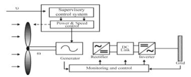
Fig. 2: Variable Speed Type Wind Energy Conversion
