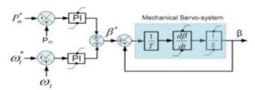
Fig. 6: Pitch Angle Control Scheme Using PI Controllers
