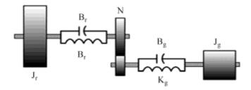
Fig.7: Two Mass Drive Train Model
