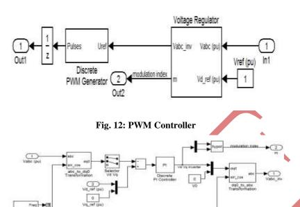
Fig .13: Voltage Controller
