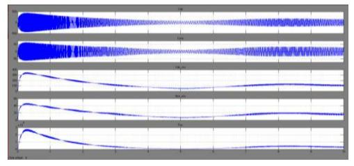
Fig. 24: Waveform Of Line To Line Voltage (Vab), Line Current (IL), Rms Line Voltage (Vab\_Rms), AC
