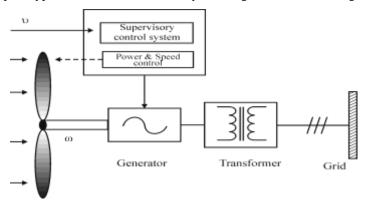
Fig. 1: Fixed Speed Type Wind Energy Conversion System
